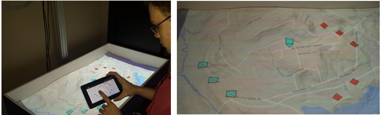
Figure 20. An example ARES scenario showing entity locations, terrain features and tactical overlays. The ARES system also provides a tablet interface to facilitate authoring.
