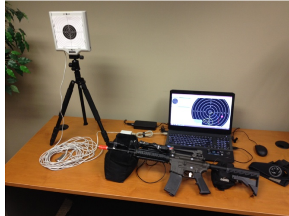
Figure 1. The experimental system: Pictured from left to right are the target, the simulated weapon, a laptop running the marksmanship program, and the physiological sensor system.
